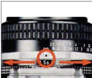
2. Set the lens to the desired f-number. Although each number on the lens aperture ring has a click stop, you can also set the ring to intermediate settings. Note that small apertures give greater depth of field, while large apertures restrict the zone of sharp focus to the main subject. The shutter speed dial can be set at any position except M250 and B
