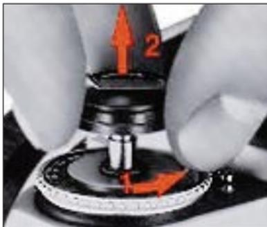
1. **Open the camera back** (40) While pushing the camera back locking lever (58) counterclockwise, pull up the film rewind knob (54) until the camera back pops open.
