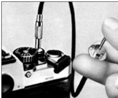
Trip the shutter by pushing the shutter release button all the way down; apply light but steady pressure with the ball of your index finger to avoid camera shake which might result in blurred images.
