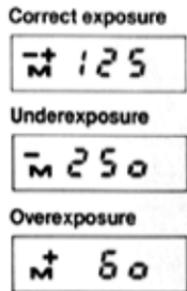
4. **Center your main subject in the viewfinder and check the exposure information.** Remember that in the manual mode, centerweighted metering is always in operation regardless of the position of the metering control button. The selected f-number is shown through the ADR window. When the shutter release button is depressed halfway, the LCD shows the selected shutter speed preceded by the letter M.
