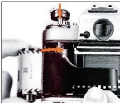
2. **Insert the film cartridge.** Position the cartridge in the film cartridge chamber (27) with the leader pointing towards the takeup spool (36); then push the rewind knob back down to secure the cartridge in place. You can use any type of 35mm film on the market. It is advisable to handle film in the shade to avoid direct exposure to sunlight.
