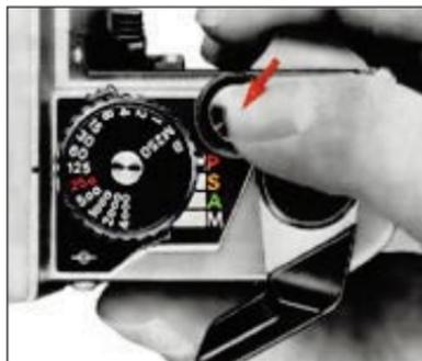
2. Depress the shutter release button halfway to activate the exposure meter.
