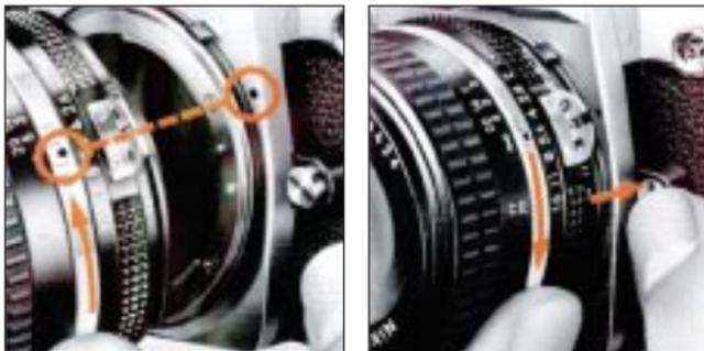
Lenses usable with the Nikon FA are AI-S Nikkor, Nikon Series E, AI-Nikkor, most AI-modified, and certain special lenses shown at the right. First line up the aperture/distance index (44) on the lens with the lens mounting index (15) on the camera body. Then twist the lens mounting ring (46) counterclockwise until the lens clicks into place. Confirm that the aperture/distance index is exactly at the top.
