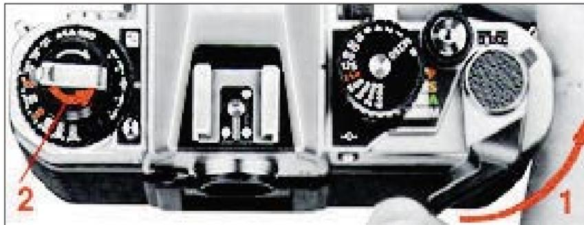
7. **Make blank exposure.** To dispose of the first few frames exposed during film loading, continue to alternately advance the film and depress the shutter release button until the frame counter (71) reaches frame 1. While making blank exposures, check that the rewind knob is rotating, indicating the film has been loaded correctly and is being advanced. If the knob does not rotate, reload the film.
