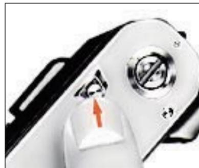
2. Depress the rewind button <sup>33</sup> on the bottom of the camera. You don't have to apply continuous pressure to the button; just press it once.
