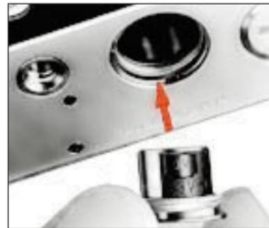
3. **Reattach the battery clips.** Slip the clip back into the camera body and screw it tightly into place.
