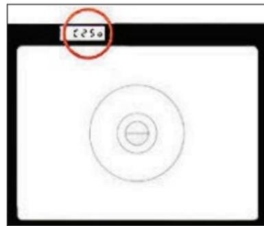
3. Check the LCD. Confirm that the LCD (liquid crystal display) is shown at the upper left in the viewfinder. This indicates that battery installation is correct and power is sufficient. If necessary, replace with a new set.
