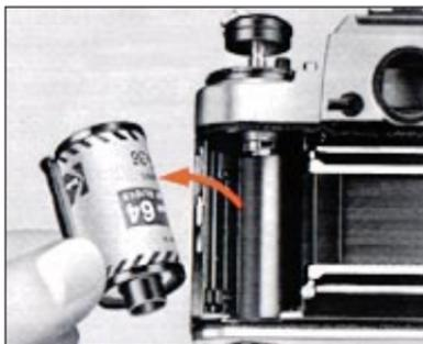
4. **Open the camera back and take out film cartridge.** Avoid unloading in direct sunlight. If there is no shade available, turn your back to the sun and use your own shadow to shield the camera.
