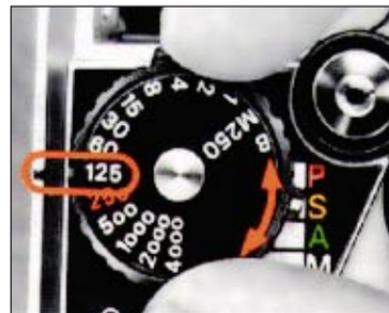
3. Set the shutter speed dial to the desired shutter speed. The numbers on the dial are reciprocals, e.g., 4000 means 1/4000sec. The 250 engraved in red indicates the fastest sync speed for an electronic flash unit. Each setting has a click stop. Shutter speeds from 1 to 1/4000sec. are electromagnetically controlled while the FA's shutter is mechanical controlled at M250 and B.
