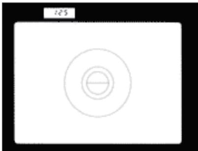
4. **Look through the viewfinder and check the exposure information.** Depress the shutter release button halfway and you will see the LCD showing the shutter speed (as a reciprocal) selected by the camera to provide correct exposure. Note that a slow shutter speed results in blurred images (techniques for avoiding blurred images are explained on page 46).
