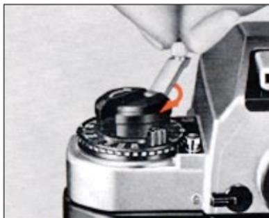
3. **Rewind the film** unfolding the film rewind crank and turning it in the direction of the arrow. When you feel the tension lessen, give it a few more turns until crank turns freely, indicating the film leader is rewound completely back into the cartridge.
