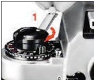
6. **Take up film slack.** Fold out the film rewind crank (57) and rotate gently in the direction of the arrow on the film rewind knob until you feel a slight resistance. Then fold the crank back in.
